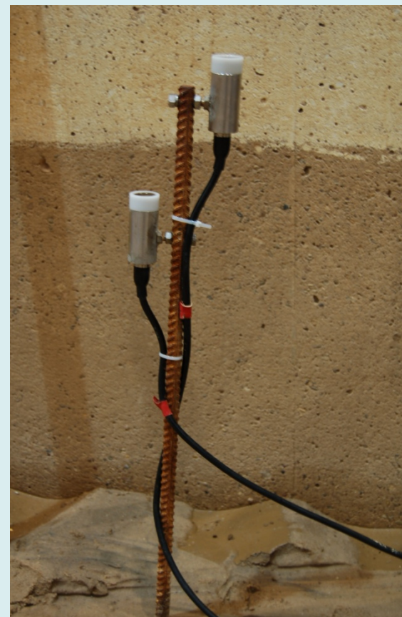
Installed as pore pressure sensor (before placed in the sand bed)
