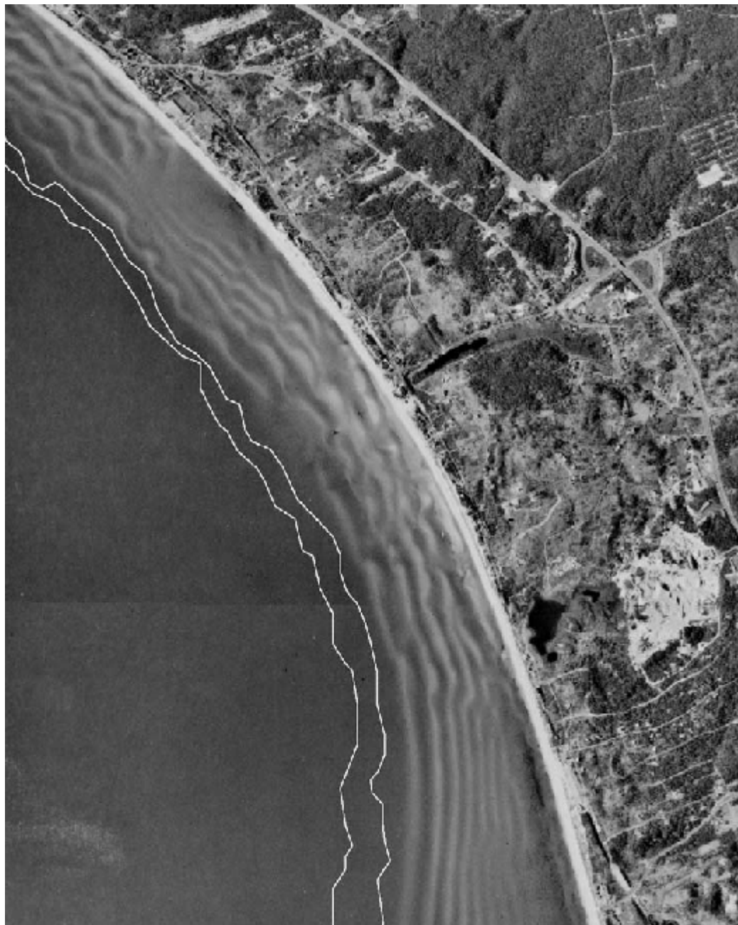
11. Multiple-bar system in Truro, Massachusetts, Cape Cod Bay (Moore et al., 2003)
